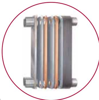
RNC Series models 25–3000 incorporate heat exchangers crafted from multiple offset layers of press formed AISI 316 stainless steel. Press forming creates peaks and valleys that form media channels that optimize fluid turbulence. This prevents fouling and maximizes energy efficiency.
